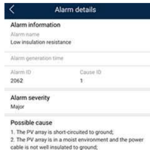
Figure E-1 Alarm details
