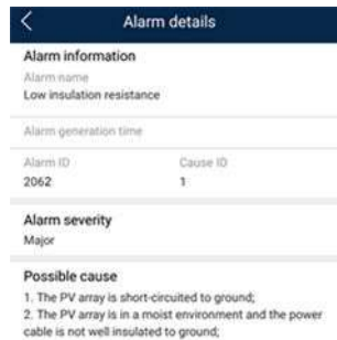
Figure E-1 Alarm details
