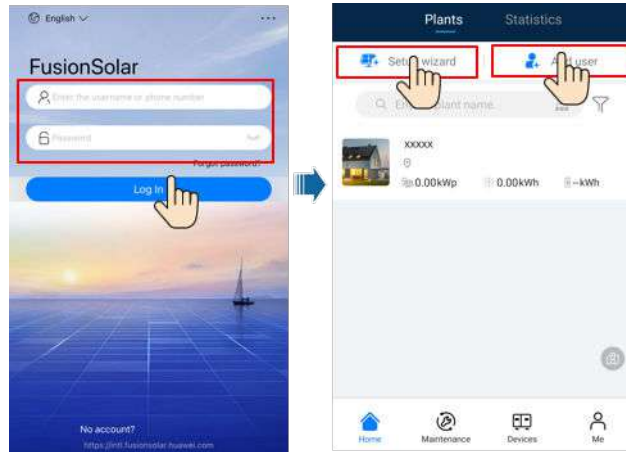
Figure 7-5 Creating a PV plant and a user
